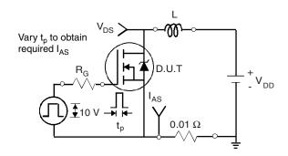
Fig. 15 - Unclamped Inductive Test Circuit
