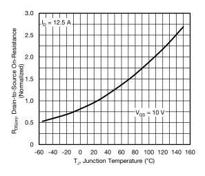
Fig. 4 - Normalized On-Resistance vs. Temperature
