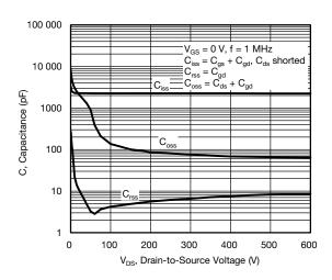
Fig. 5 - Typical Capacitance vs. Drain-to-Source Voltage
