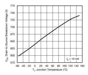
Fig. 11 - Typical Drain-to-Source Voltage vs. Temperature
