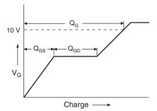
Fig. 17 - Basic Gate Charge Waveform
