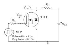
Fig. 13 - Switching Time Test Circuit
