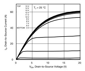
Fig. 1 - Typical Output Characteristics
