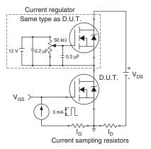
Fig. 18 - Gate Charge Test Circuit
