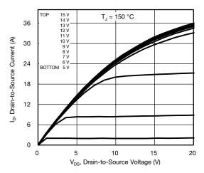
Fig. 2 - Typical Output Characteristics
