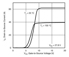
Fig. 3 - Typical Transfer Characteristics
