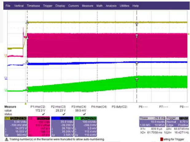
CH1: V CC , CH2: V DRAIN , CH3: V LED , CH4: I LED
