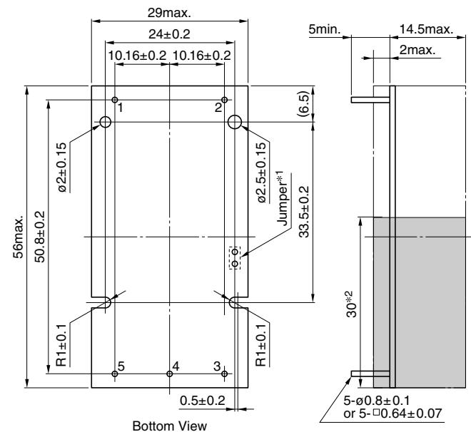
\*1 Terminal numbers 2 and 5 are connected by the jumper.
