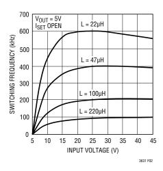
Figure 2. Switching Frequency for  $V_{OUT} = 5V$
