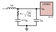
Figure 5. Series RC to Reduce VIN Ringing
