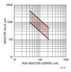
Figure 4. Recommended Inductor Values for Maximum Efficiency
