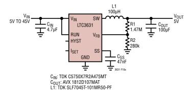
Figure 10. High Efficiency 5V Regulator
