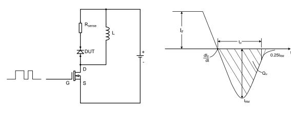
t<sub>rr</sub> Test Circuit
