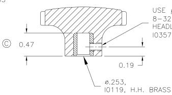
USE #28 DRILL, 8-32 TAP,  $8-32 \times 1/4$  LG. CUP POINTED, HEADLESS, SLOTTED SET SCREW, 10357, (1) REQ'D
